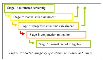
Each of the first 4 stages represents an escalation in contingency and the fifth stage capitalizes the lessons learned. Basically, information provided by external databases is recorded and processed by in-house tools that screen the collision risks and produce collision assessments that are gradually refined. Eventually, an avoidance maneuver is considered. Figure 2 shows the global information flow of this process.
