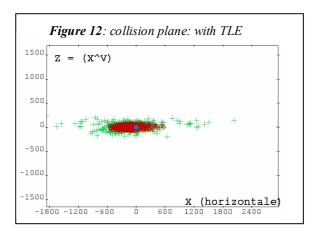
The following action was the computation of the operational probability of collision. In our current example this probability was equal to 2.5 10<sup>-3</sup>. This figure was greater than 10<sup>-3</sup>, which was another reason for the CA team to ask for radar measurements in order to improve the orbit knowledge of the debris.
